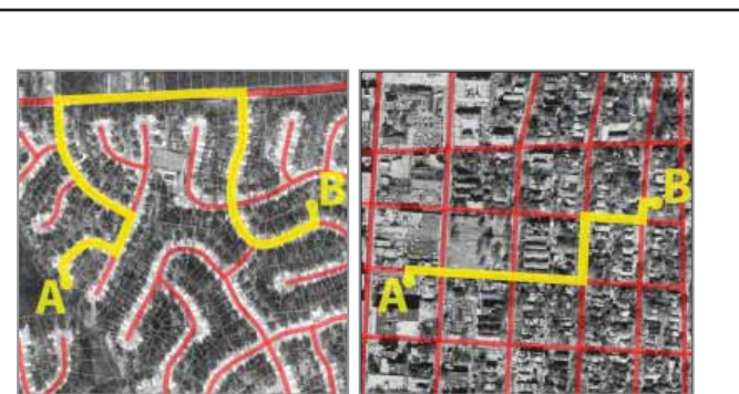
Dendritic system: the distance from A to B is one mile and achievable along one route Interconnected system: the distance from A to B is one half mile with multiple route options
